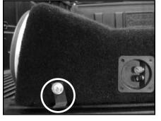
**STEP 6**Secure the other L-bracket to the right side of the Stealthbox\*.
